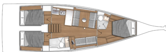
FIRST 44 interior – 3 cabins / 2 heads
