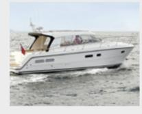
Max. length: Approx. 11,8 m Max. beam: Approx. 3,5 m Draught: Approx. 1,1 m Approx. 7000 kg Weight: Cruising speed: 15-28 knots Type of hull: Semi-planing Material: Vacuum infused GRP - Vinylester Air draft: 2,95 m (without navigation mast) Volvo Penta D6 330-480 HP V-gear Engine: Diesel: Approx. 600 L Water: Approx. 300 L Holding: Approx. 150 L CE-category: C Manufactured in: Norway
