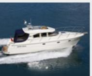
Max. length: 12,63 m 3,92 m Max. beam: 8.000 kg Weight: Type of hull: Semi-planing with deep keel Vacuum infused GRP Material: Air draft: 4.55 m Volvo Penta D6 330-435 HPS V-gear Engine: Cruising speed 15-18 knots 1000 L Diesel: 525 L Water: Holding: 230 L CE-category: B Manufactured in: Norway
