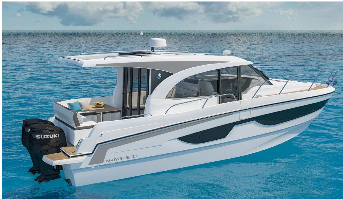
The new Antares has twin outboard engines (2 x 300 CV/HP maximum engine power) to guarantee performance and comfort.
